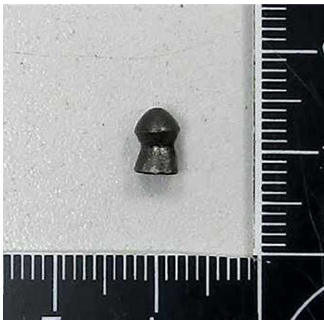
ryc 4. The cal. 4.5. 'Diabolo Boxer' projectile, made in the Czech Republic, intended for pneumatic weapons and devices, extracted from a gunshot wound to the victim's chest and used as evidence.
