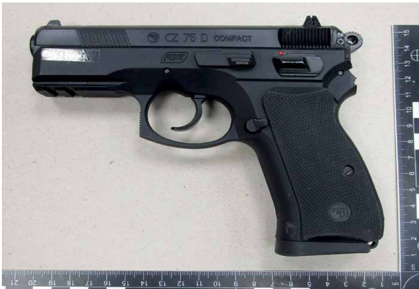
ryc 1. The cal. 4.5 mm CZ 75 D Compact ASG pneumatic pistol, made in Taiwan, provided for testing.
