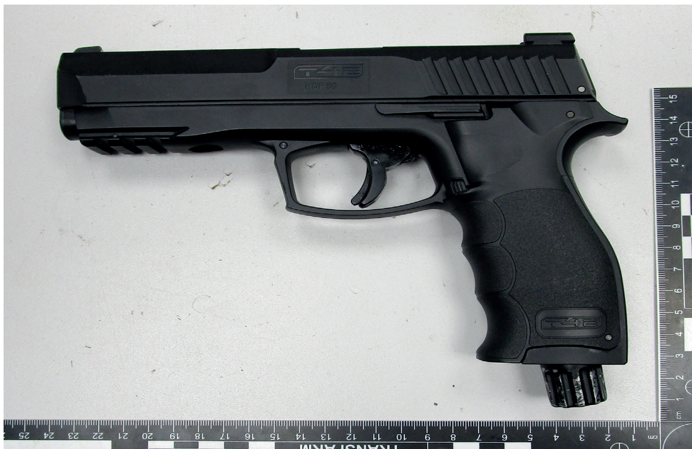
ryc 5. The cal. 12.7 mm (50'') Umarex T4E HDP 50 pneumatic pistol, made in Germany, provided for testing.
