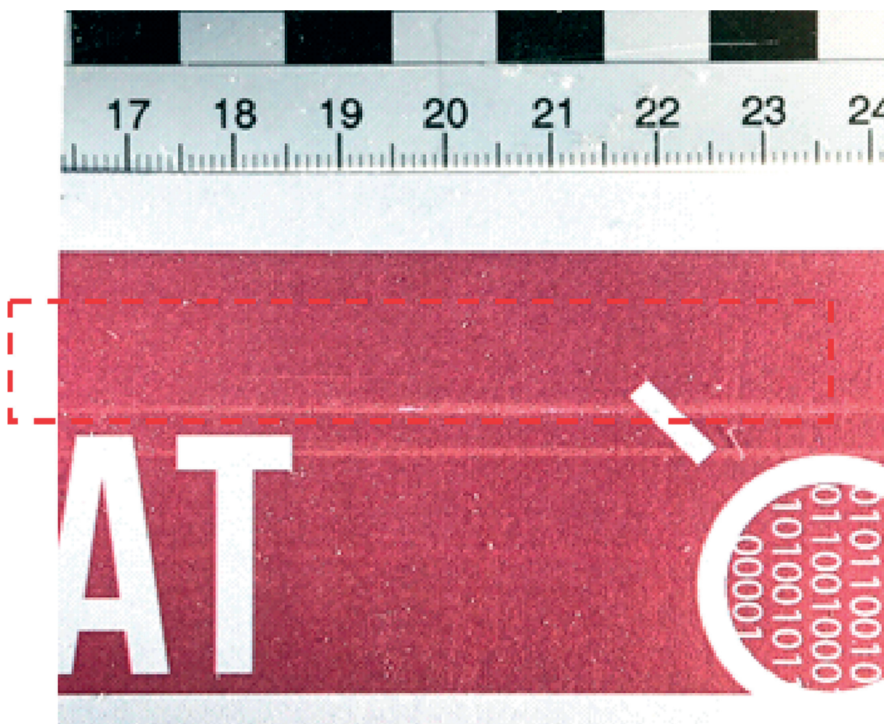
ryc. 10. Traces on the printout applied by a malfunctioning paper tear-off device. Source: the authors.
