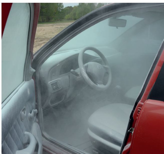
ryc. 12 The car interior after using the fire extinguisher.
