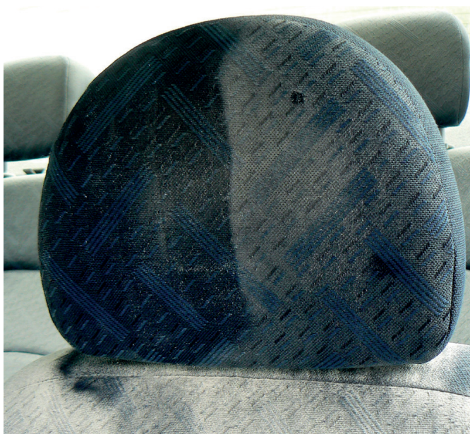
ryc. 15 The headrest after mechanical and manual removal of the fire extinguishing powder.
