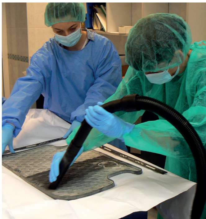
ryc. 6 Removal of the extinguishing powder with a vacuum cleaner - the rubber floor mat.
