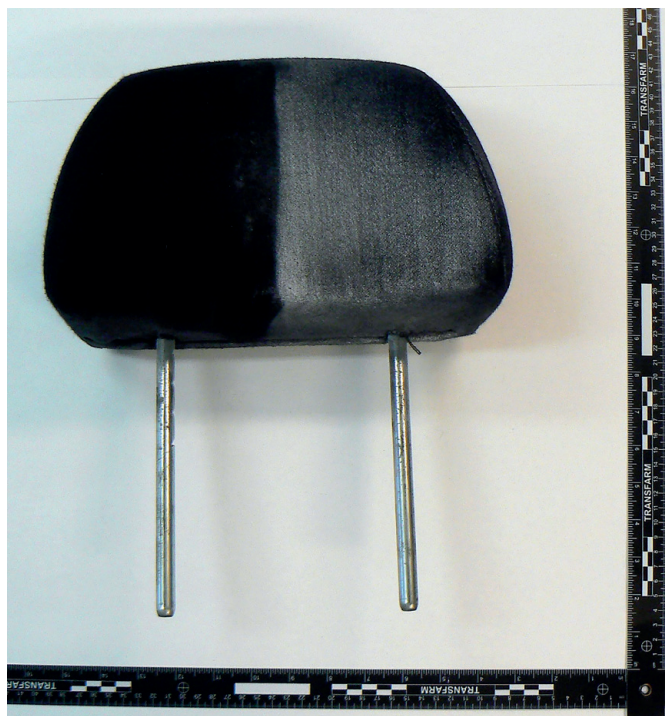
ryc. 5 The headrest after mechanical and manual removal of the fire extinguishing powder.
