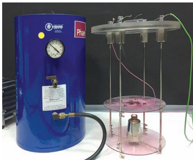
Fig. 2. Chamber utilized in the studies, dedicated to the cyanoacrylate method, adapted for sublimation of other substances.
