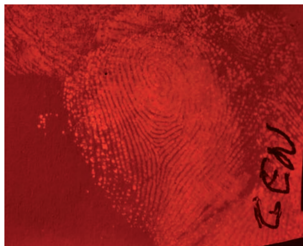
Fig. 4. Fingerprints revealed using genipin vacuum sublimation technique – a view in the fluorescence mode (excitation 575 nm, red longwave edge filter).
