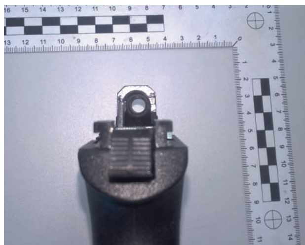
Fig. 10. View of the ZORAKI pistol barrel after disassembling the plug from the muzzle.
