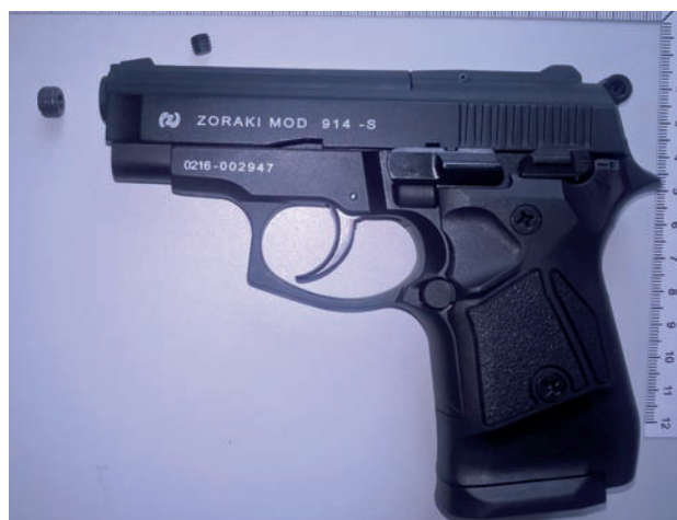
Fig. 2. Side view of ZORAKI mod. 914-S cal. 9 mm P.A. pistol (with the detached plug).
