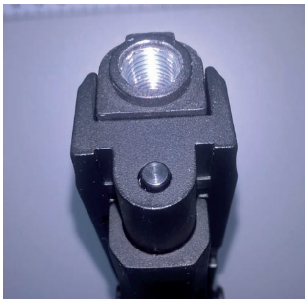
Fig. 5. Threaded muzzle of ZORAKI mod. pistol 914-S cal. 9 mm P.A.
