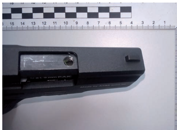
Fig. 3. Threaded hole in the upper flat of the barrel of the ZORAKI mod. 906 cal. 9 mm P.A. pistol
