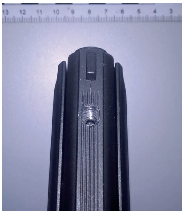
Fig. 4. Threaded hole in the upper wall of the barrel of the ZORAKI mod. 914-S cal. 9 mm P.A. pistol
