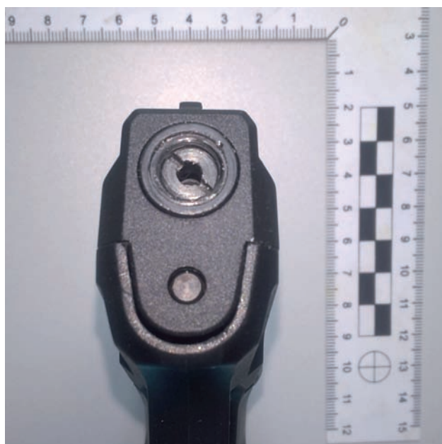
Fig. 8. Plug with central socket mounted in the muzzle of the ZORAKI mod. 906 pistol.
