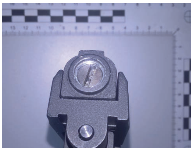
Fig. 9. Plug (without a socket) mounted in the muzzle of a ZORAKI mod. 914-S pistol.
