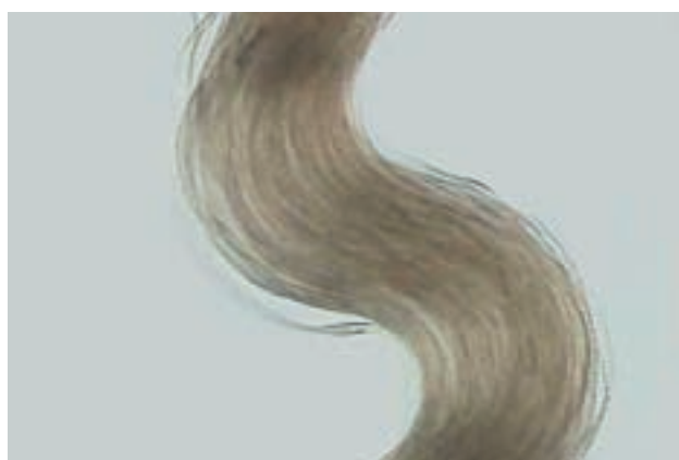
Fig. 64, 65. Appearance of single threads of polyester (100% polyester) under the research microscope, at 100x magnification. From the left: brand-new fabric, 3x laundered fabric (own material).
