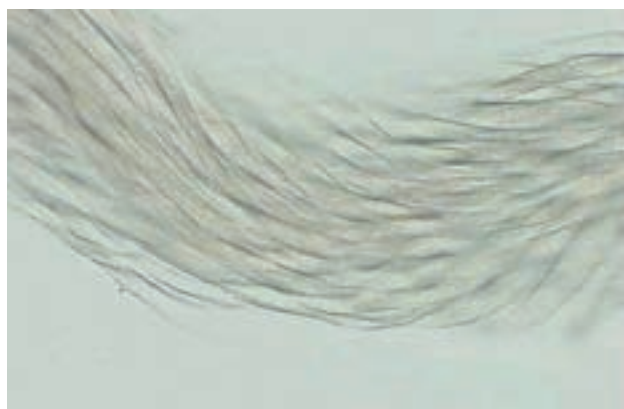
Fig. 62, 63. Appearance of single threads of asti wool (60% wool, 40% polyester) under the research microscope, at 100x magnification. From the left: brand-new fabric, 3x laundered fabric (own material).
