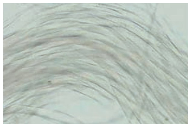
Fig. 62, 63. Appearance of single threads of asti wool (60% wool, 40% polyester) under the research microscope, at 100x magnification. From the left: brand-new fabric, 3x laundered fabric (own material).
