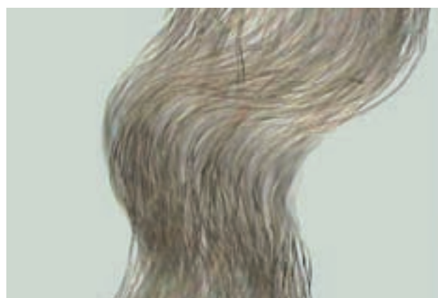
Fig. 64, 65. Appearance of single threads of polyester (100% polyester) under the research microscope, at 100x magnification. From the left: brand-new fabric, 3x laundered fabric (own material).
