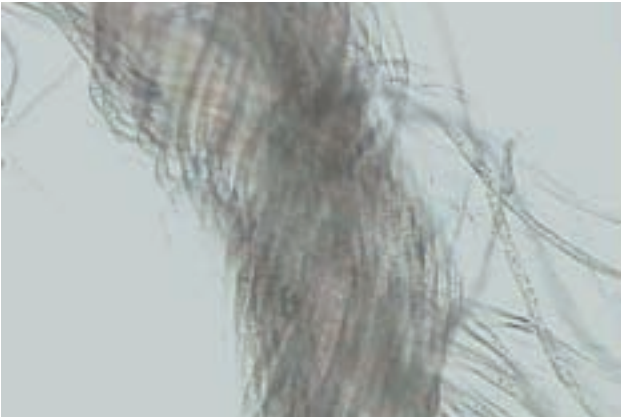
Fig. 58, 59. Appearance of single threads of massimo viscose (52% viscose, 45% polyester, 3% spandex) under the research microscope, at 100x magnification. From the left: brand-new fabric, 3x laundered fabric (own material).
