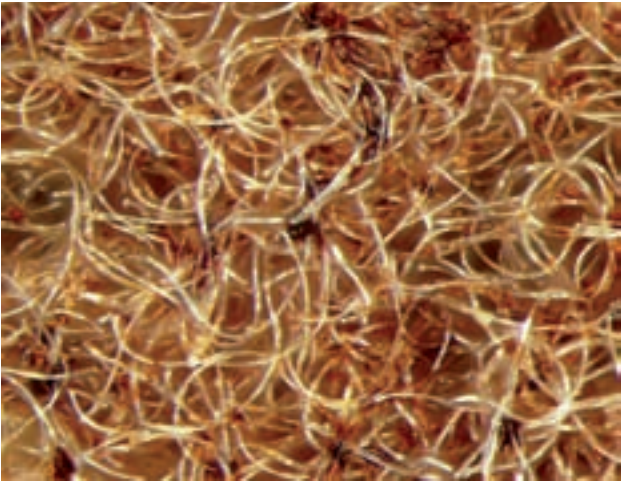
Fig. 36. Closeup on the structure of a bloodstained polar fabric at 163x magnification (own elaboration).
