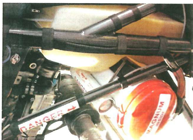
Fig. 7. Rescue system mounted on a paraglider carriage. Labels clearly indicate the threat posed by the parachute rescue system.
