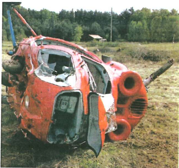
Fig. 3. Sample location of the battery pack on board the Mi-2 helicopter in front of the fuselage hatch.
