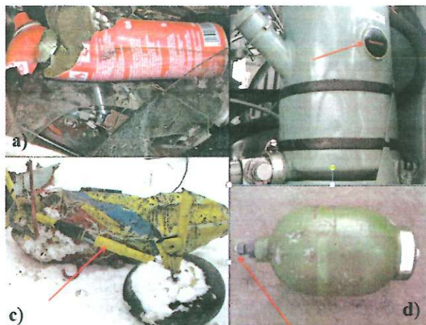
Fig. 4. Different pressure storage tanks; a) ruptured on-board fire extinguisher, b) oil tank – measuring glass indicates the level of oil, c) main landing gear shock absorber helicopter, d) a compressed gas cylinder – charging valve.
