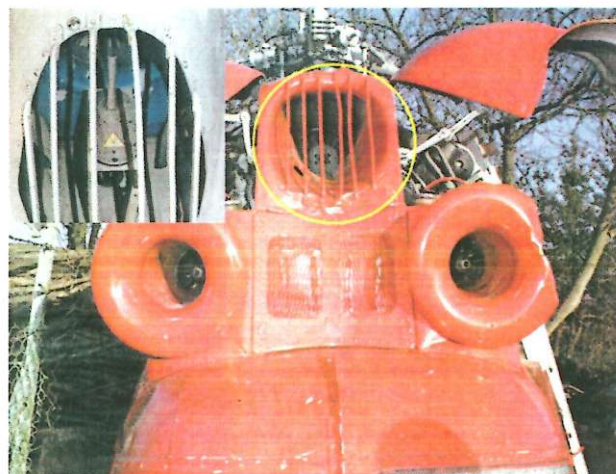
Fig. 5. Location of the dismantled icing siren on a Mi-2 helicopter and a view of the siren, clearly marked as a source of radioactive radiation.
