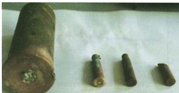
Fig. 8. The cases of disassembled cartridges after cleaning.
