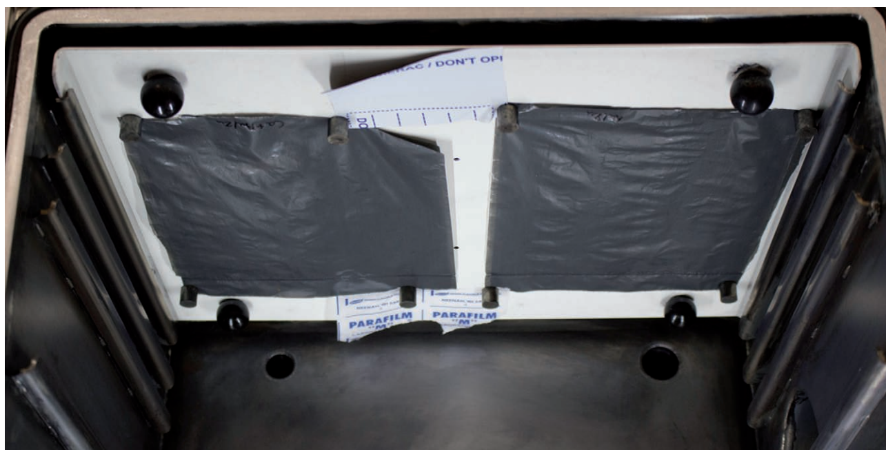
Fig. 7. The manner of mounting exhibits for the visualization process: surfaces to be treated are held with magnets in the upper part of VMD360 chamber in a special mount.
