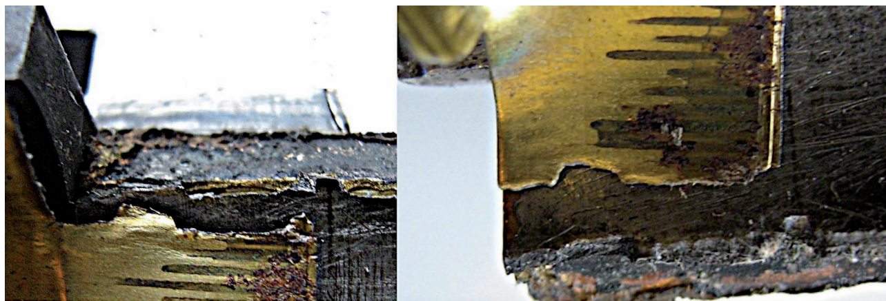
Fig. 4. View of the folded edges of the ruptured cartridge chamber and cartridge shell.
