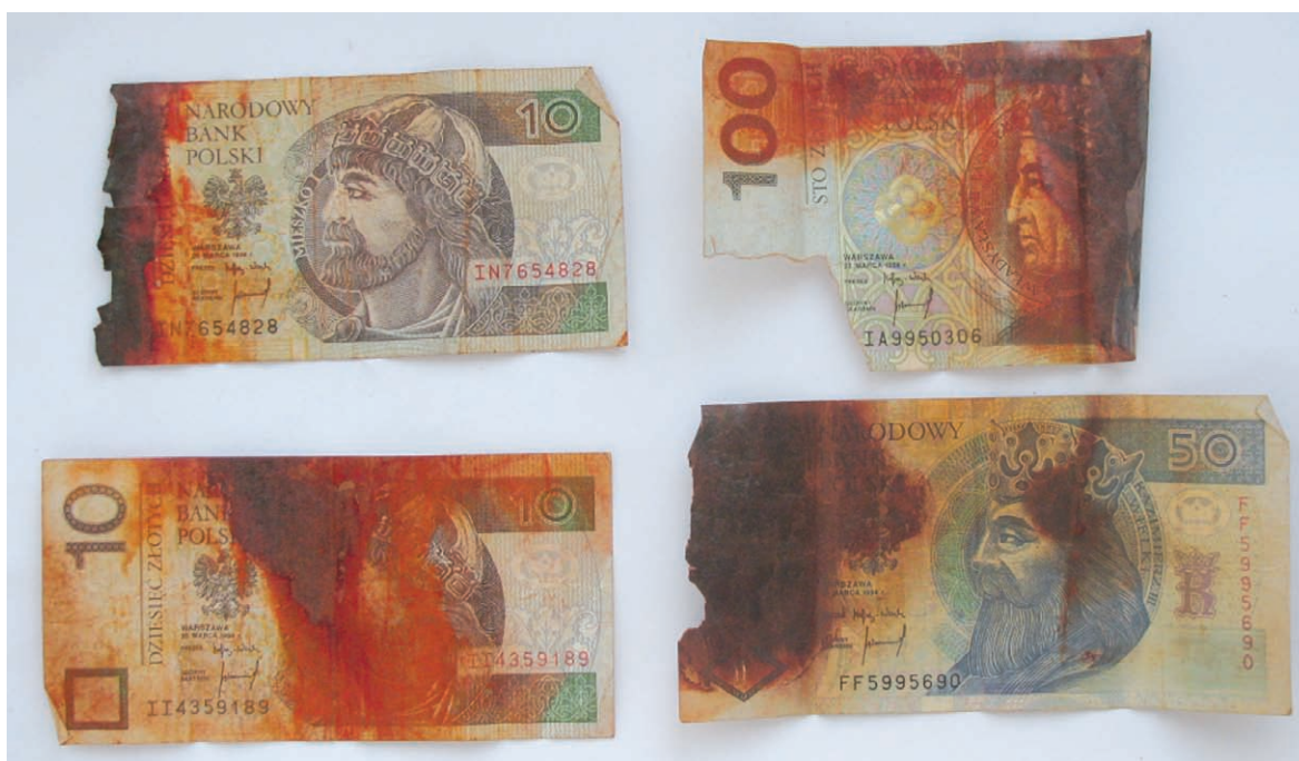
Fig. 15. Banknotes damages by smoke generator of the anti-theft device (dye used: quinizarine).
