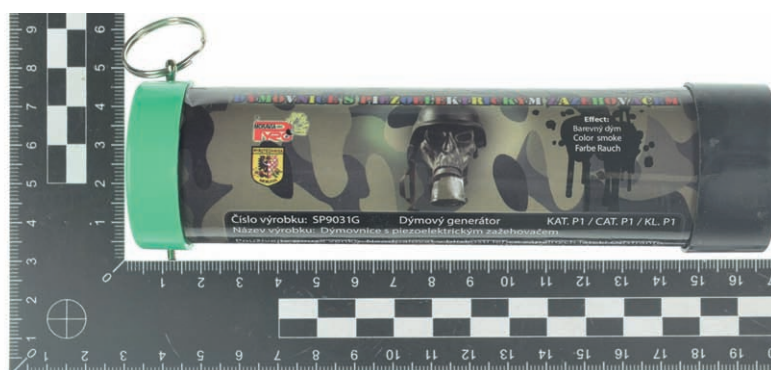
Fig. 5. Smoke generator with a piezoelectric ignition system.
