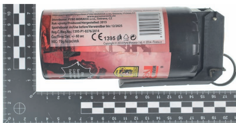
Fig. 6. Smoke generator with a friction igniting system and a trigger lever.
