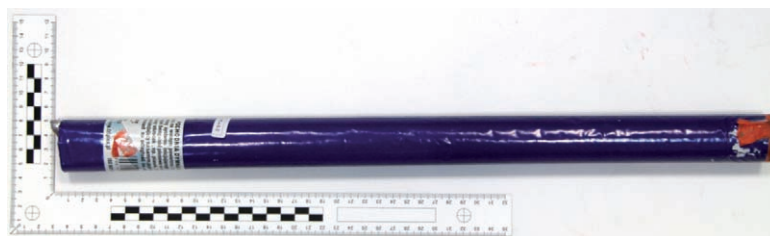
Fig. 4. Generator of blue smoke with a fuse initiating system.
