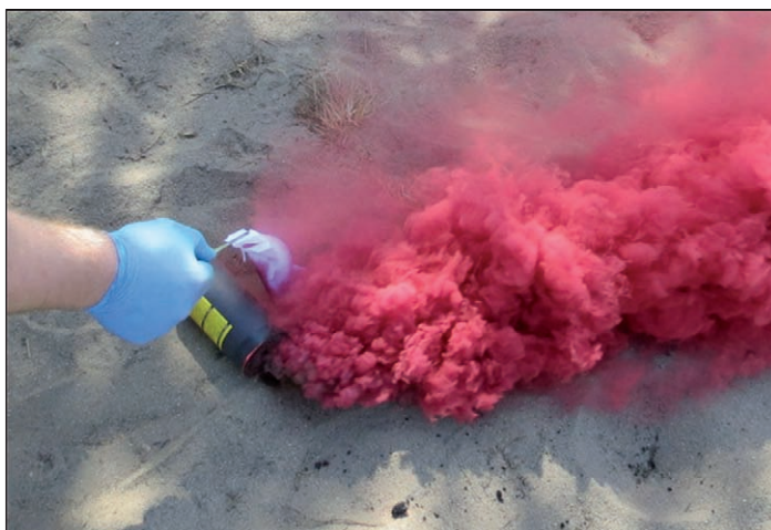
Fig. 7. Collection of analytical sample from a stream of smoke.
