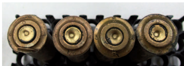
Fig. 5. Case bottoms from 11 mm × 60R calibre Mauser rifle cartridges fired in the course of weapons proficiency tests. Visible traces of the firing pin and manufacturer's markings.
