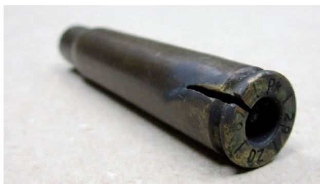
Fig. 7. Damaged case of the fired 7.92 × 57 mm calibre Mauser rifle cartridge from 1929, manufactured in Poland.
