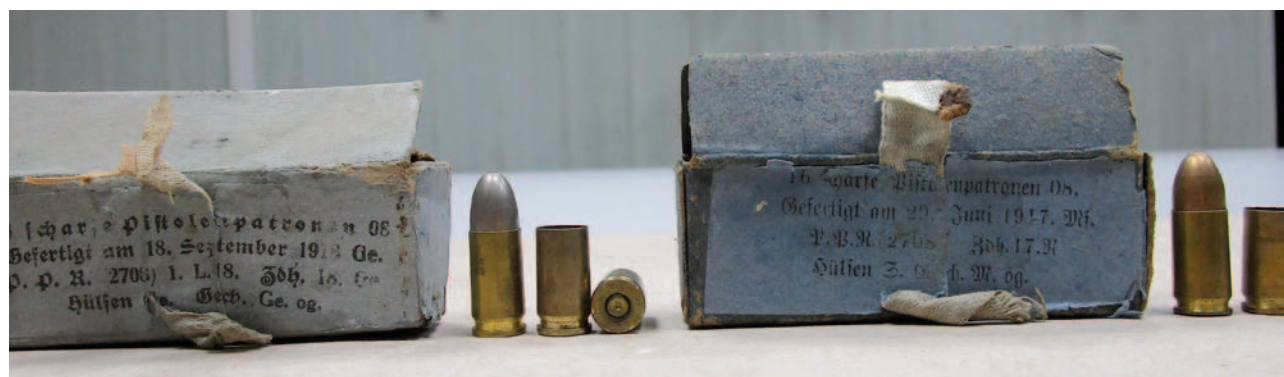
Fig. 1. Parabellum 9 x 19 mm calibre pistol cartridges from 1917 and 1918 submitted for testing and cartridge cases from evidence cartridges fired with ammunition packaging. The bullet jackets of the cartridges from the packaging dated 18 September 1918 were melchior-clad, while the remaining cartridges had bullets with tombac-clad jackets.
