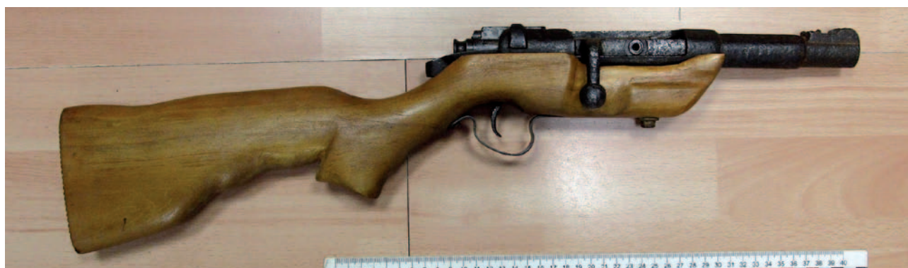
Fig. 2. Single-shot Mauser Model 1871 11 mm calibre rifle, without numbers, produced by Germany, in the condition as submitted for testing, the so-called “sawn off”.
