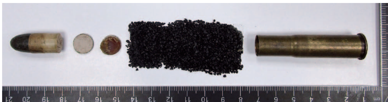
Fig. 3. Disassembled 11 mm × 60R calibre Mauser Model 1878 rifle cartridge: a bullet with a paper wrap, a cardboard attachment, a wax and a cardboard (bottom) attachment, black (smoky) gunpowder, a case.
