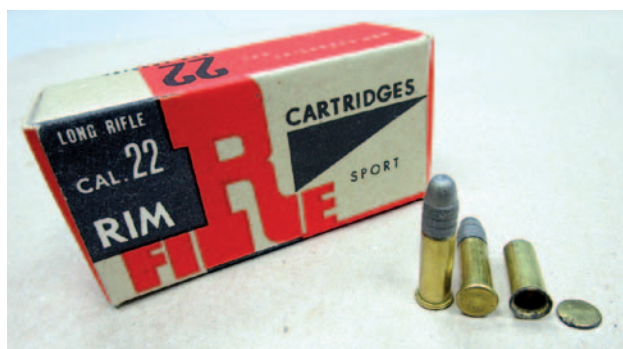
Fig. 6. “Regular SPORT rim fire cartridges” from the 1970s, which are nowadays the cause of dangerous case ruptures during firing. Next to the cartridges, there is a ruptured case in the form of a body and a detached bottom. Ammunition packaging is shown in the background.
