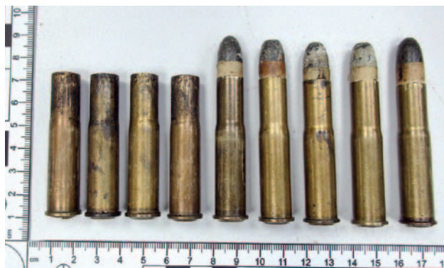
Fig. 4. 11 mm × 60R calibre Mauser rifle cartridges and cases thereof after being fired from the Mauser Model 1871 11 mm calibre rifle, without numbers, manufactured in Germany.
