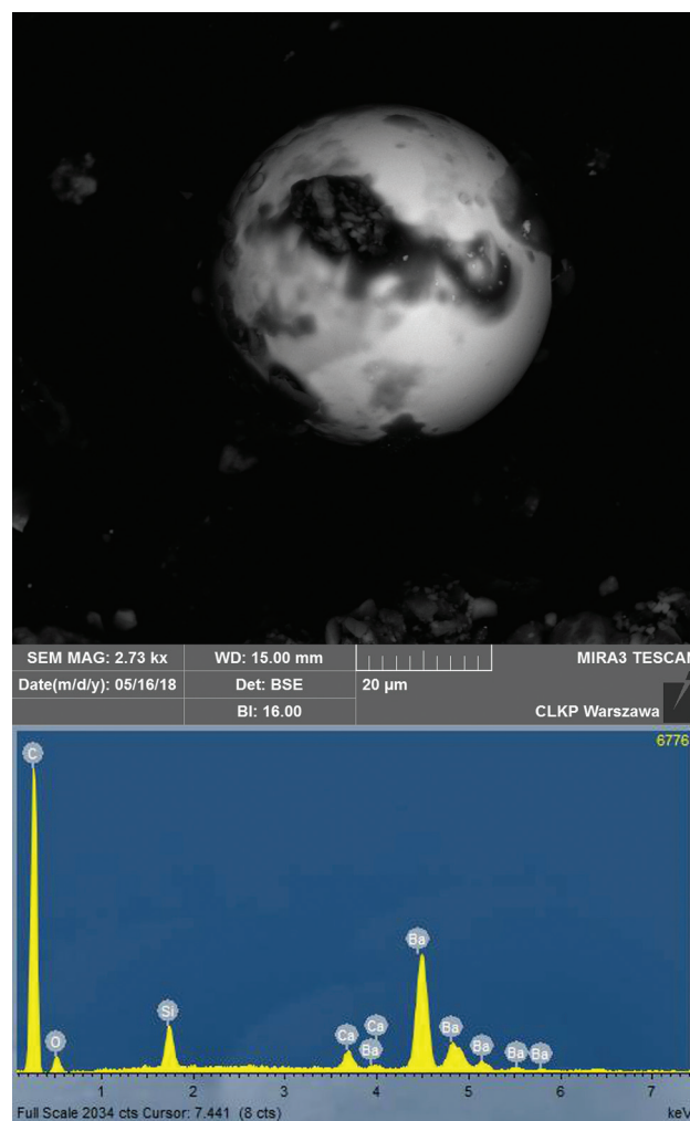
Fig. 7. Image and EDX spectrum of BaCaSi particle detected on car backseat and denominated with K17 code.
