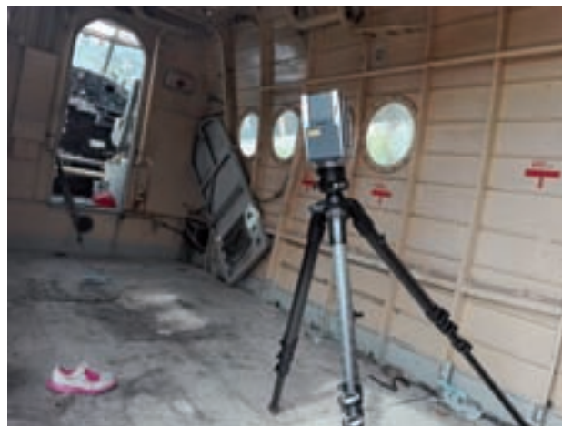
Fig. 5. 3D laser scanning.
