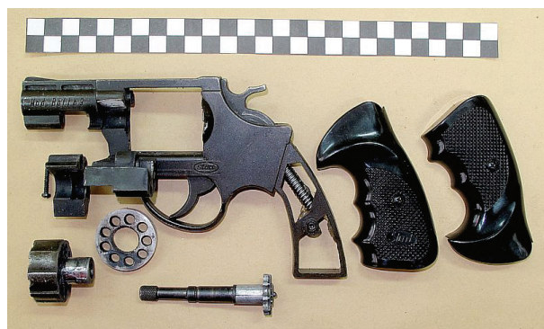
Fig. 10. Exemplary design of a converted alarm revolver: a partition was removed from the barrel bore; a blind part of the cylinder was cut off, while simultaneously attaching a disc with six holes.
