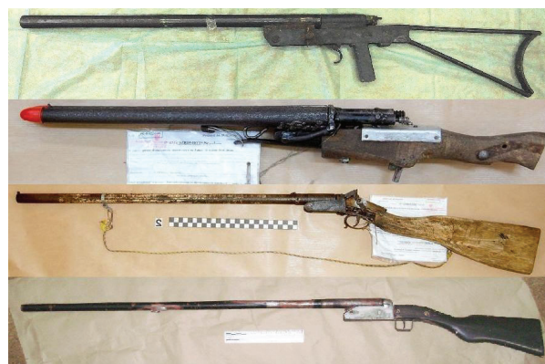
Fig. 1. Improvised shotguns compatible with hunting ammunition.
