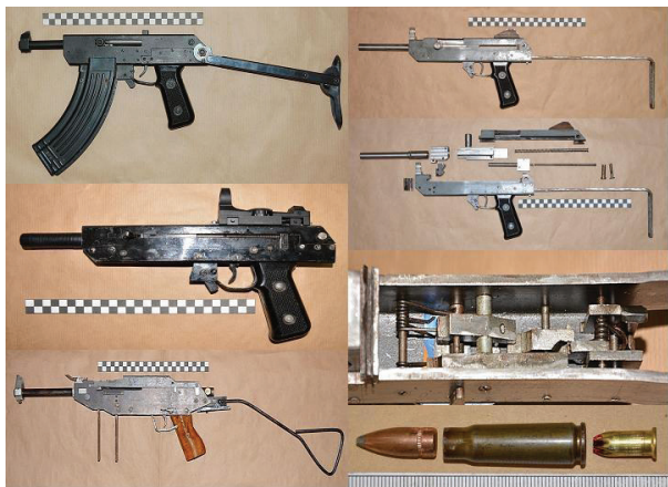
Fig. 6. Improvised submachine guns (one piece disassembled, offering a detailed view of the mechanism) and improvised ammunition.
