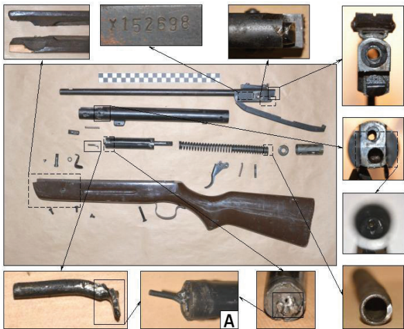
Fig. 7. Exemplary design of an improvised pneumatic weapon: reamed compressed air outlet channel; a thin metal rod welded to the compression piston serves as the firing pin (A).
