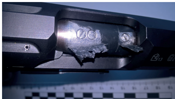
Fig. 5. View of barrel pinholes closed with screws.
