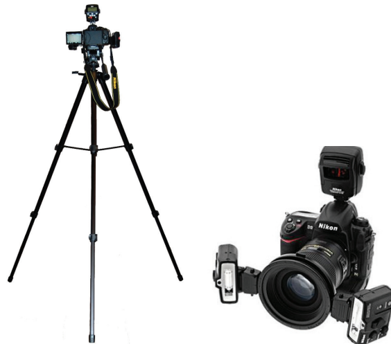
Fig. 3. Nikon D5300 camera on a tripod, supplemented with a set of wireless flash lamps to perform macro photography.
