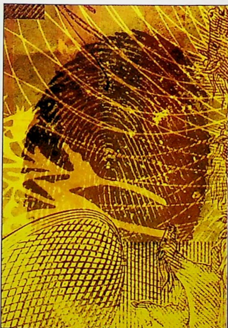
Ryc. 16. Ślad z ryc. 15 ujawniony safraniną po wymyciu Basic Yellow 40 (505 nm – filtr 550 nm) Fig. 16. Mark from Fig. 15 developed with saphranine following washing off Basic Yellow 40 (505 nm, 550 nm filter)
