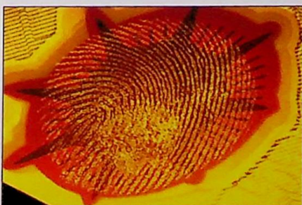
Ryc. 19. Ślad z ryc. 18 ujawniony safraniną po wymyciu Basic Yellow 40 (505 nm – filtr 550 nm) Fig. 19. Fingerprint from Fig. 18 developed with saphranine after washing off Basic Yellow 40 (505 nm, 550 nm filter)
