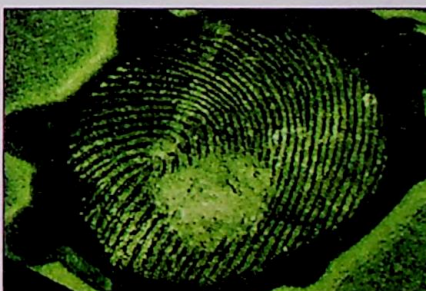
Ryc. 20. Ślad z ryc. 19 ujawniony proszkiem BVDA B-47950 po wymyciu safraniny (350 nm – filtr 475 nm) Fig. 20. Fingerprint from Fig. 19 developed with BVDA B-47950 powder after washing off saphranine (350 nm, 475 nm filter.)
