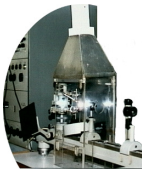
Fig. 1. A spectrograph stand with electrodes mounted on it (a UBI-1 generator can be seen in the background)
