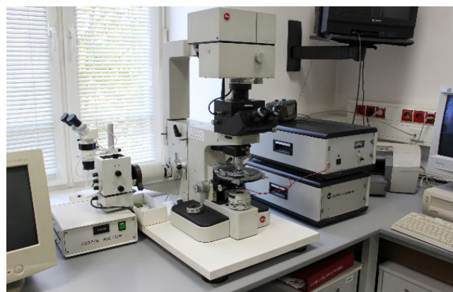
Fig. 15. A UV-VIS microspectrophotometer
