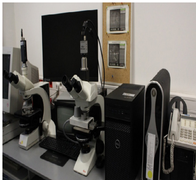
Fig. 11. A refractive index measurement kit GRIM III
