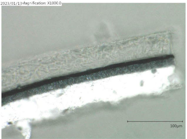
Fig. 9. A microscopic image of a cross-section of a paint coating under white light (BF)
