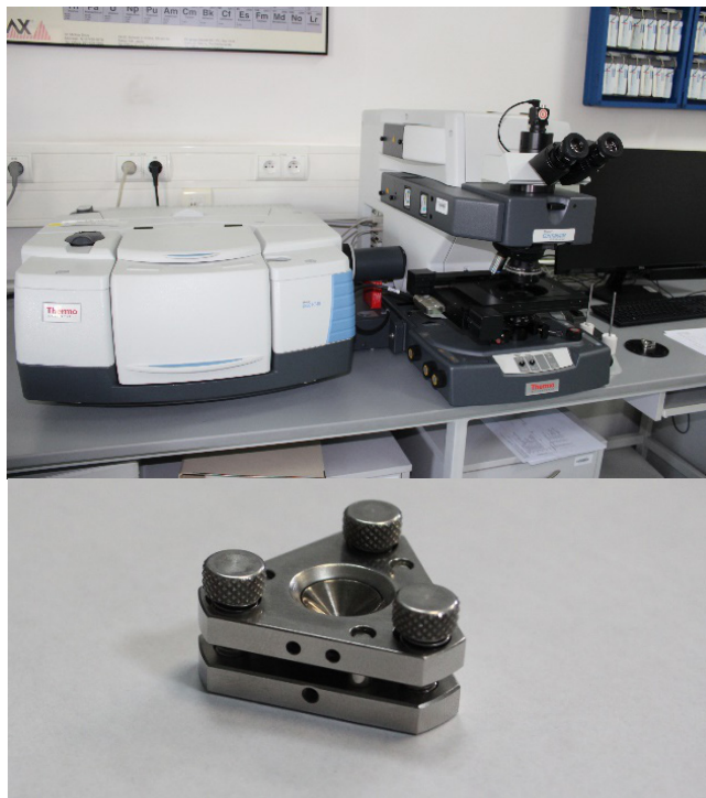
Fig. 13, 14. Fourier-transform infrared spectroscopy with a diamond cell
