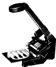
Fig. 3. Zeiss SP 2 spectroprojector (without the outer casing and curtains)
