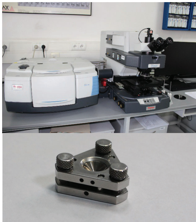
Fig. 13, 14. Fourier-transform infrared spectroscopy with a diamond cell
