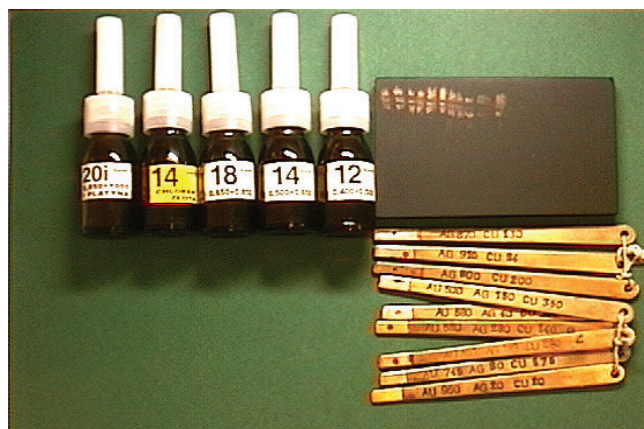
Fig. 9. A test kit for determining fineness of precious metal products
