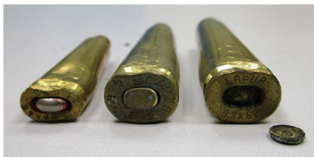
Photo 4. View of the cartridge case heads crushed laterally in the vice jaws. The bottom of the primer cup of the Finnish-made 9.3×62 mm hunting rifle cartridge case has come off. The primers did not fire
