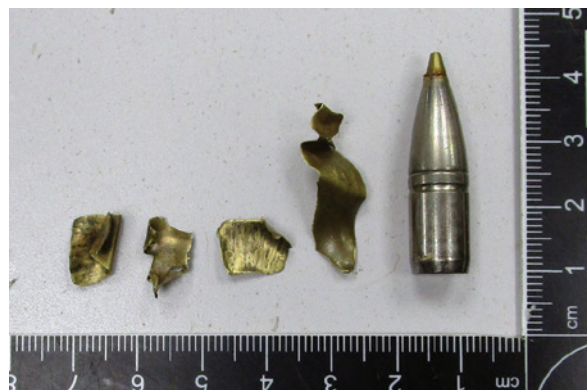
Photo 2. The questioned bullet recovered from the injured man's body and the fragments of the ruptured cartridge case found at the scene
