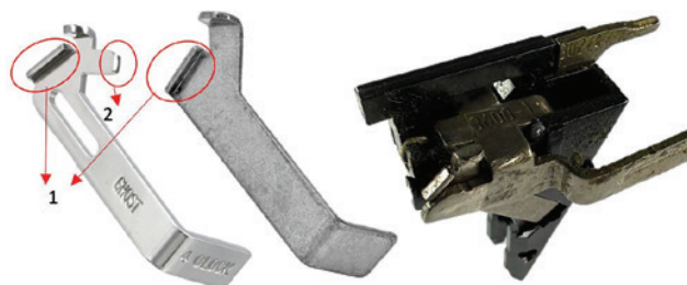
Fig. 6. From left: GHOST connector, source: https://besthunters.pl/ accessed on 26 August 2026, where 1 – the surface along which the trigger bar moves; 2 – TCT, Trigger Control Tab. Factory connector, source: https://coltwroclaw.pl/ accessed on 26 August 2026; part of the trigger mechanism showing the trigger bar and the connector surface along which it moves (mechanism fitted with the factory connector)
