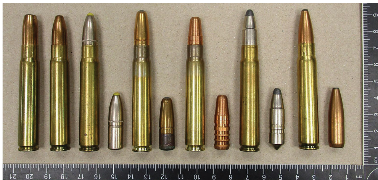
Photo 3. 9.3×62 mm hunting rifle cartridges of various manufacturers (from left): Sellier & Bellot, Norma, Norma with a “Plastic Point” bullet, Lapua with a “Mega” bullet, Lapua with a “GPA” bullet, RWS with a “TUG” bullet, T with an “SP” bullet
