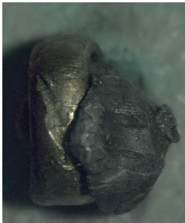
Fig. 7. Traces of the barrel rifling marks on the evidence submitted primer and on the piece of the projectile
