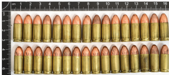
Fig. 5. Pistol ammunition – general view, showing the crimping points securing the bullet in the case
