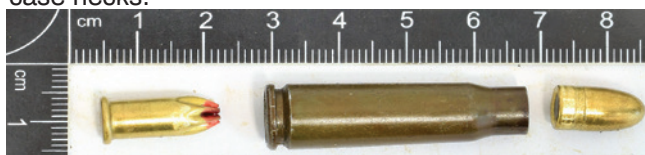
Fig. 16. Submachine gun ammunition – view of the components
