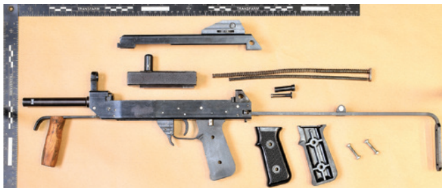
Fig. 8. Submachine gun – general view from the left side, disassembled into its main parts
