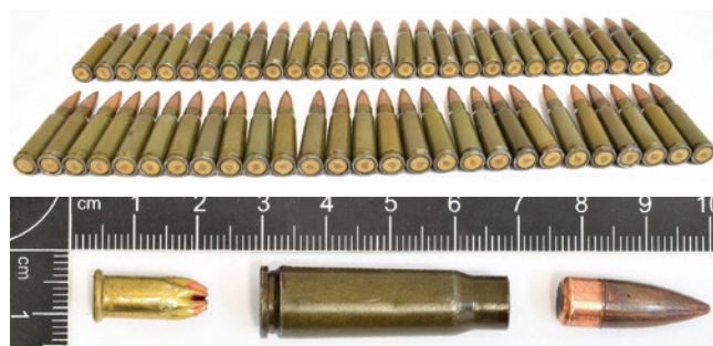
Fig. 14, 15. Submachine gun ammunition – general view and components
