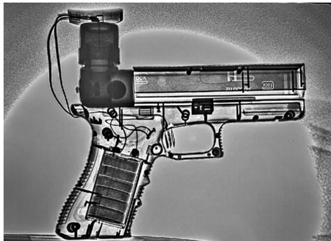
Fig. 2. A homemade cal. 15 mm pistol – an X-ray image
