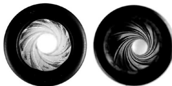
Fig. 1. Polygonal rifling, Gen 3 (left) – Marksman Barrel rifling, Gen 5 (right), authors' own work
