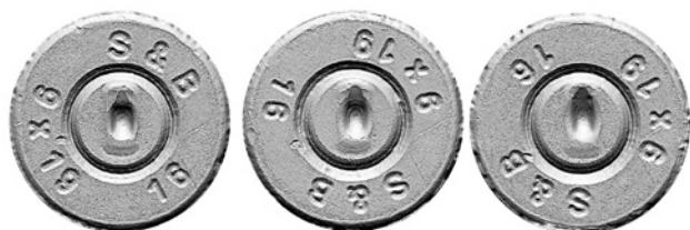
Fig. 1. Cartridge cases fired from three different Glock 17 pistols. From left: pistol No. 1, No. 2 and No. 3
